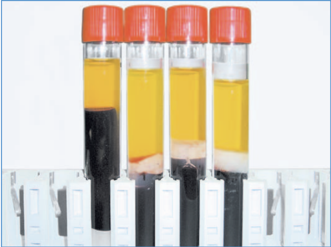
Fig. 25: Incorrectly centrifuged serum sep tubes: the wrong centrifugation speed has been applied. From left to right, the effects of an increasingly higher g-force. On the right, a correctly centrifuged serum sep tube.
